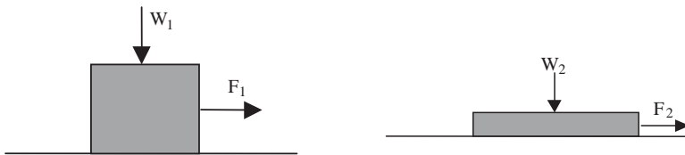
Figure 7.17 The frictional forces on two objects made from the same material, placed on the same surface, are equal if they have the same weights, i.e. if W_1 = W_2 then F_1 = F_2
